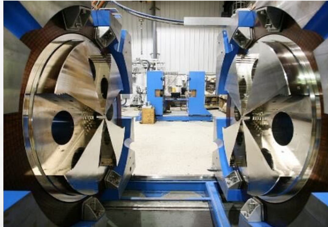
Medical purpose cyclotron
