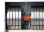
Existing SPS bunch compression cavity. The flanges of the CR DR will be very similar to this cavity.
