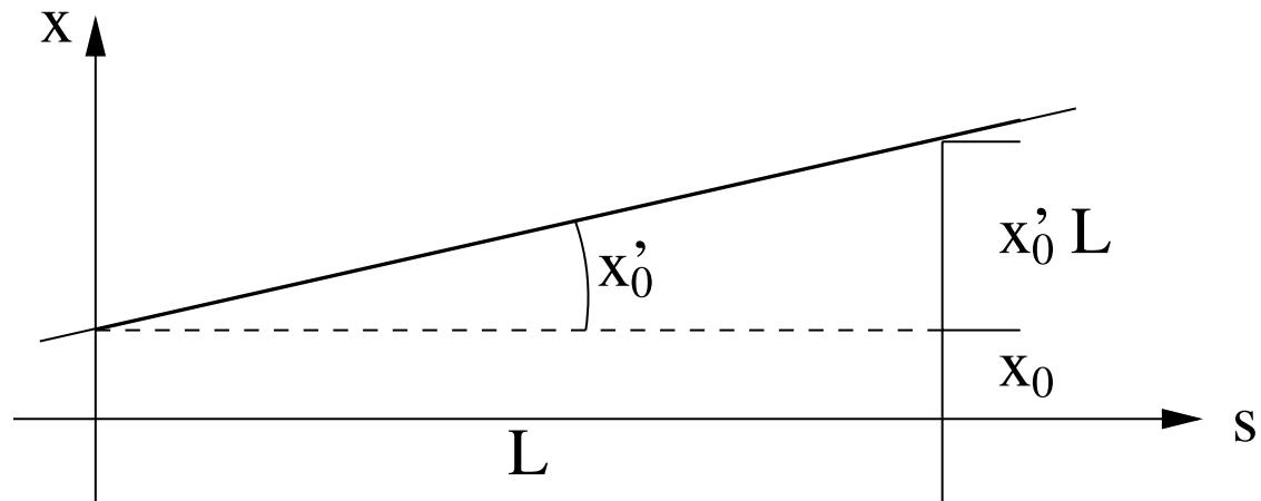
$$\mathbf{R}_{\text{drift}} = \begin{bmatrix} 1 & L & 0 & 0 & 0 & 0 \\ 0 & 1 & 0 & 0 & 0 & 0 \\ 0 & 0 & 1 & L & 0 & 0 \\ 0 & 0 & 0 & 1 & 0 & 0 \\ 0 & 0 & 0 & 0 & 1 & L/\gamma^2 \\ 0 & 0 & 0 & 0 & 0 & 1 \end{bmatrix}$$
