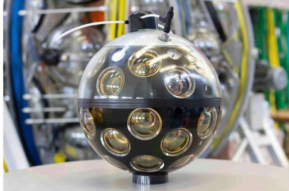
Fig. 47. The KM3NeT optical module (from reference 381). The optical module consists of a glass sphere with a diameter of 42 cm, housing 31 photosensors (yellowish disks). The glass sphere can withstand the pressure of the water and is transparent to the faint light that must be detected to see neutrinos.
