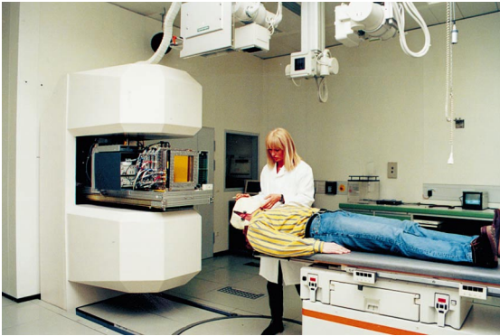
Fig. 7. A patient is prepared for a carbon ion treatment. In order to get an exact positioning of the target volume the head of the patient is fixed with an individually manufactured mask. The end of the beam pipe with ionization and multi-wire chambers for the beam control is visible at the left side. During irradiation, the PET cameras above and below the ionization chambers are placed over the patient.
