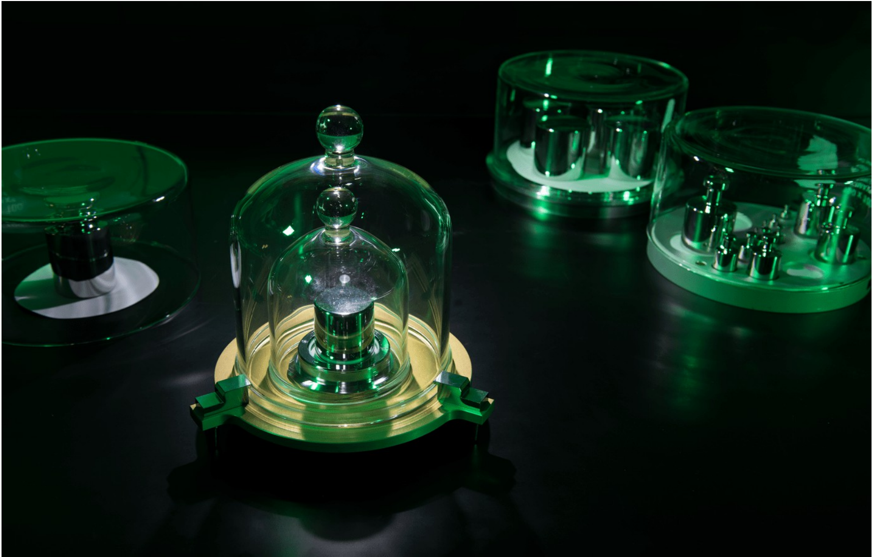
NIST's platinum-iridium kilogram K92 (front) with stainless-steel kilogram masses in the background. Credit: J.L. Lee/NIST
