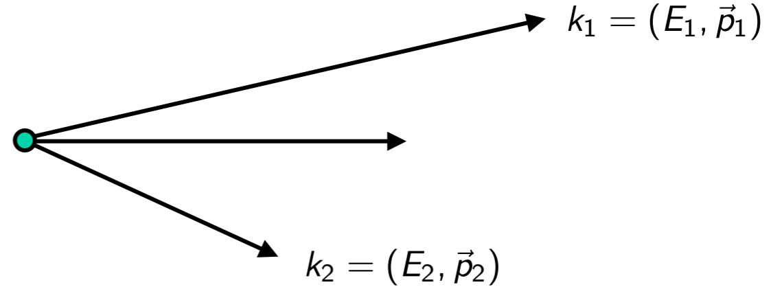
$$\begin{aligned} m^2 &= (k_1 + k_2)^2 = m_1^2 + m_2^2 + 2k_1 k_2 \\ &= m_1^2 + m_2^2 + 2E_1 E_2 - 2\vec{p}_1 \cdot \vec{p}_2 \\ &= m_1^2 + m_2^2 + 2E_1 E_2 - 2p_1 p_2 \cos \theta \end{aligned}$$
