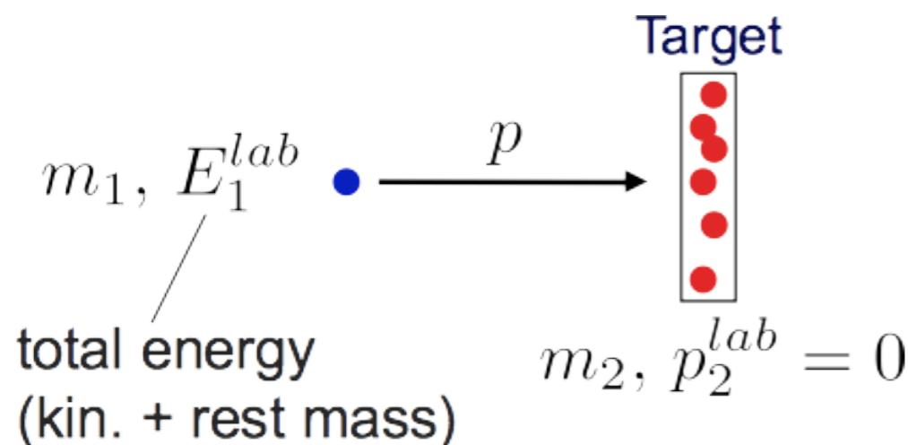
$$k_1 = (E_1^{\text{lab}}, \vec{p}_1^{\text{lab}}), \quad k_2 = (m_2, \vec{0})$$
