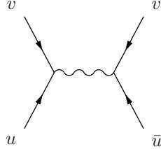
It consists of four external fermions labeled according to Tab. 1, one internal photon, and two interaction vertices. From Eq.(1.25) and Tab. 1 we know how to describe external fermions in terms of spinors.
