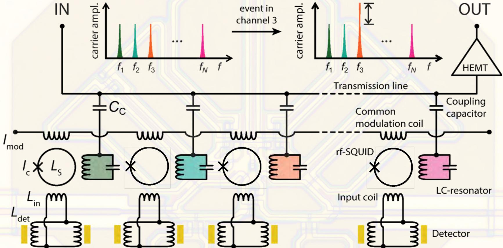
array readout using only **one** HEMT amplifier and **two** coaxes
