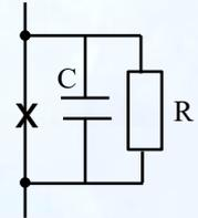
**underdamped** junction (large  $R$  and  $C$ )
