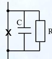
**underdamped** junction (large  $R$  and  $C$ )
