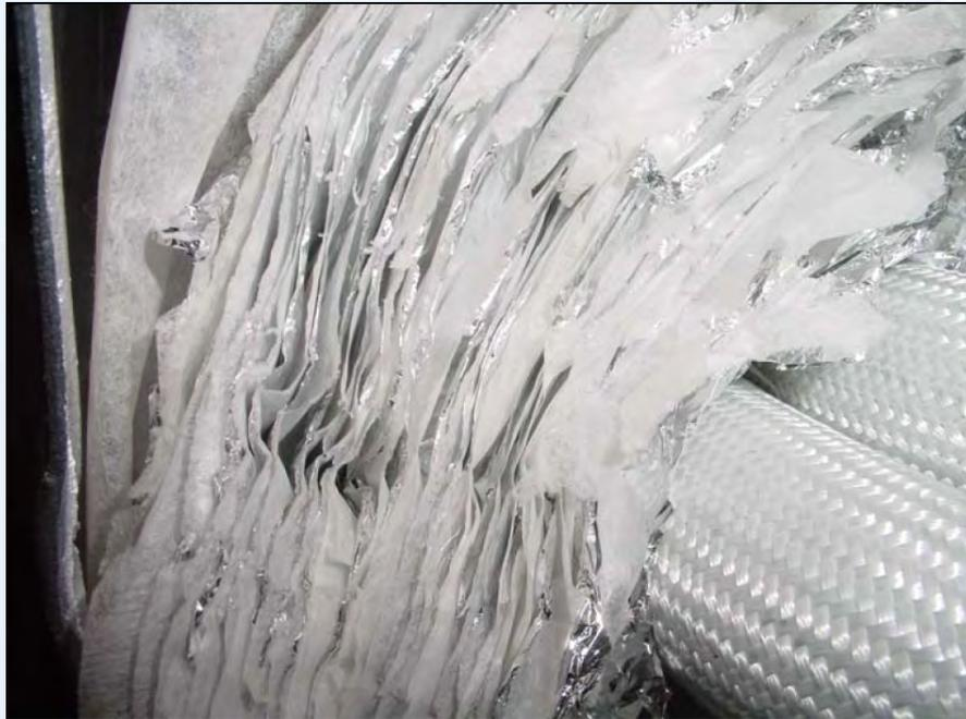
multiple radiation shields  $\rightarrow$  smaller steps  $\rightarrow$  reduction of heat flow
