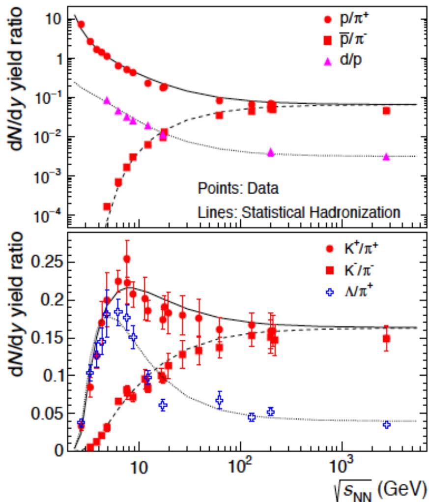
together with known energy dependence of charged hadron production in Pb-Pb collisions we can predict yield of all hadrons at all energies with < 10% accuracy
