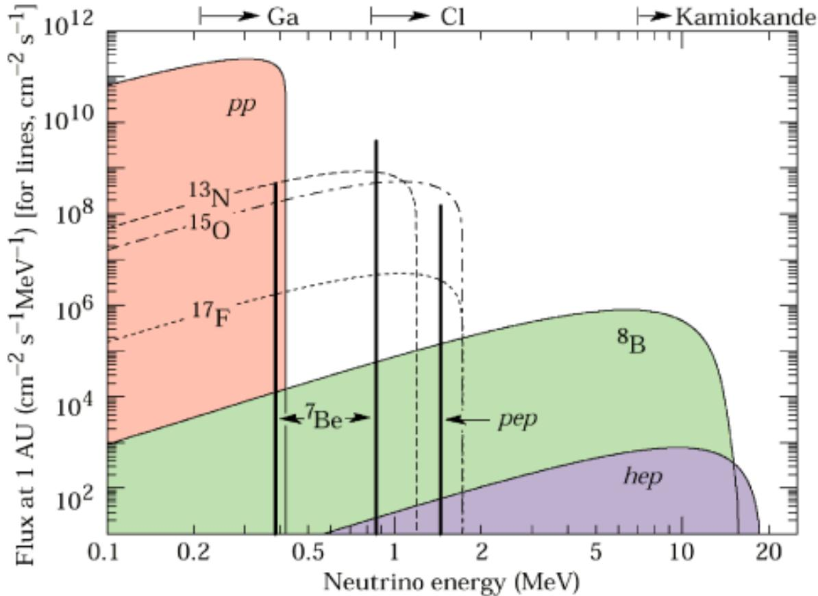
$\text{Cl}_2$  detector  $\nu_e + {}^{37}\text{Cl} \rightarrow {}^{37}\text{Ar} + e$ ,  ${}^{37}\text{Ar} \rightarrow {}^{37}\text{Cl}$  (EC)  $E_\nu > 0.8 \text{ MeV}$
