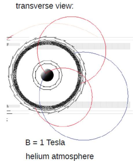
Tracking detector will consist of very thin CMOS pixel sensors to minimize multiple scattering and to optimize energy / vertex resolution.
