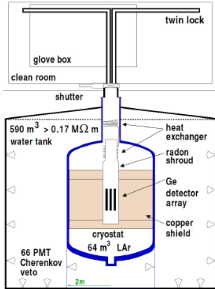
Problem: Shielding against natural radioactivity and possible radioactive pollution producing background around the end-point.
