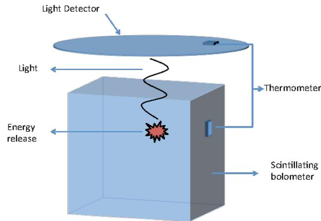
CUORE uses bolometers to search for neutrinoless double beta ( $0\nu\beta\beta$ ) decay and other rare processes. The bolometers are ultra-cold tellurium dioxide ( $\text{TeO}_2$ ) crystals containing the candidate  $0\nu\beta\beta$  isotope  $^{130}\text{Te}$ . Every time a tellurium nucleus decays or a particle interacts in the crystal, it releases a minute amount of energy (less than a few MeV), causing the temperature of the crystal to rise slightly.
