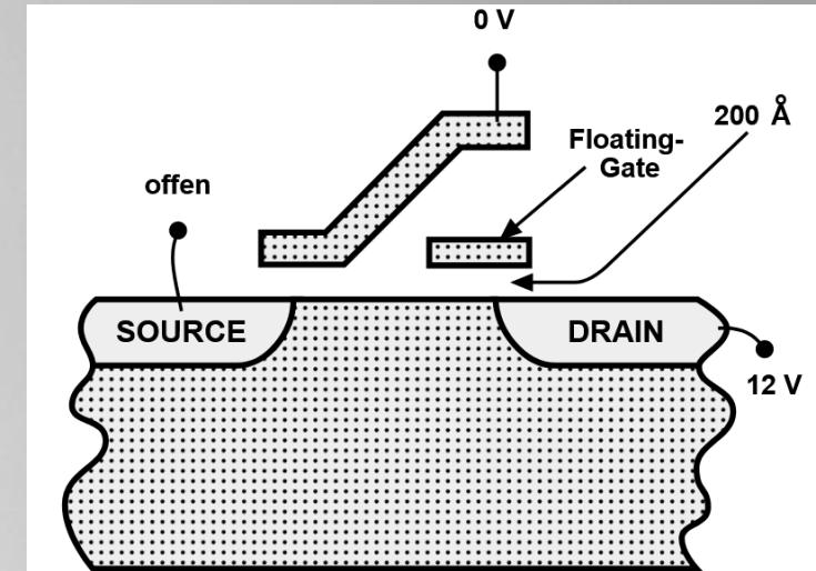
Charge in floating gate determines bit value
